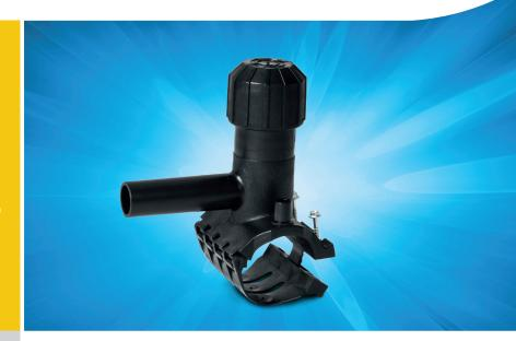
The AGRU tapping saddle creates branches on gas pipes under full pressure ("hot tapping") without interrupting the operation. This pressure tapping fitting is characterised by quick, easy and safe installation. Manufactured from stress crack-resistant PE 100-RC, the AGRU tapping saddle stands for maximum reliability during installation and subsequent operation.
